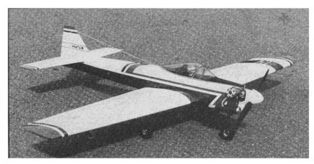
effort well worth the little extra building time required. Along the same vein, the fin was smoothly faired into the fuselage to clean up that turbulence generator.
