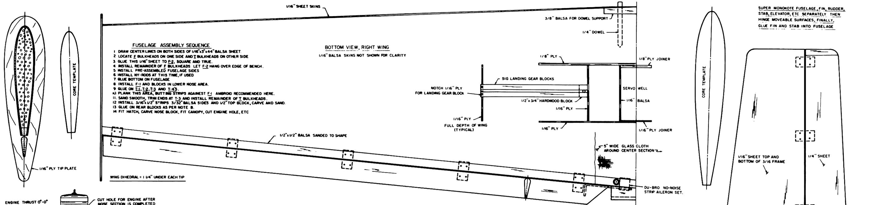
SUPER MONOKOTE FUSELAGE, FIN, RUDDER, STAB, ELEVATOR, ETC. SEPARATELY, THEN HINGE MOVEABLE SURFACES, FINALLY, GLUE FIN AND STAB INTO FUSELAGE.
