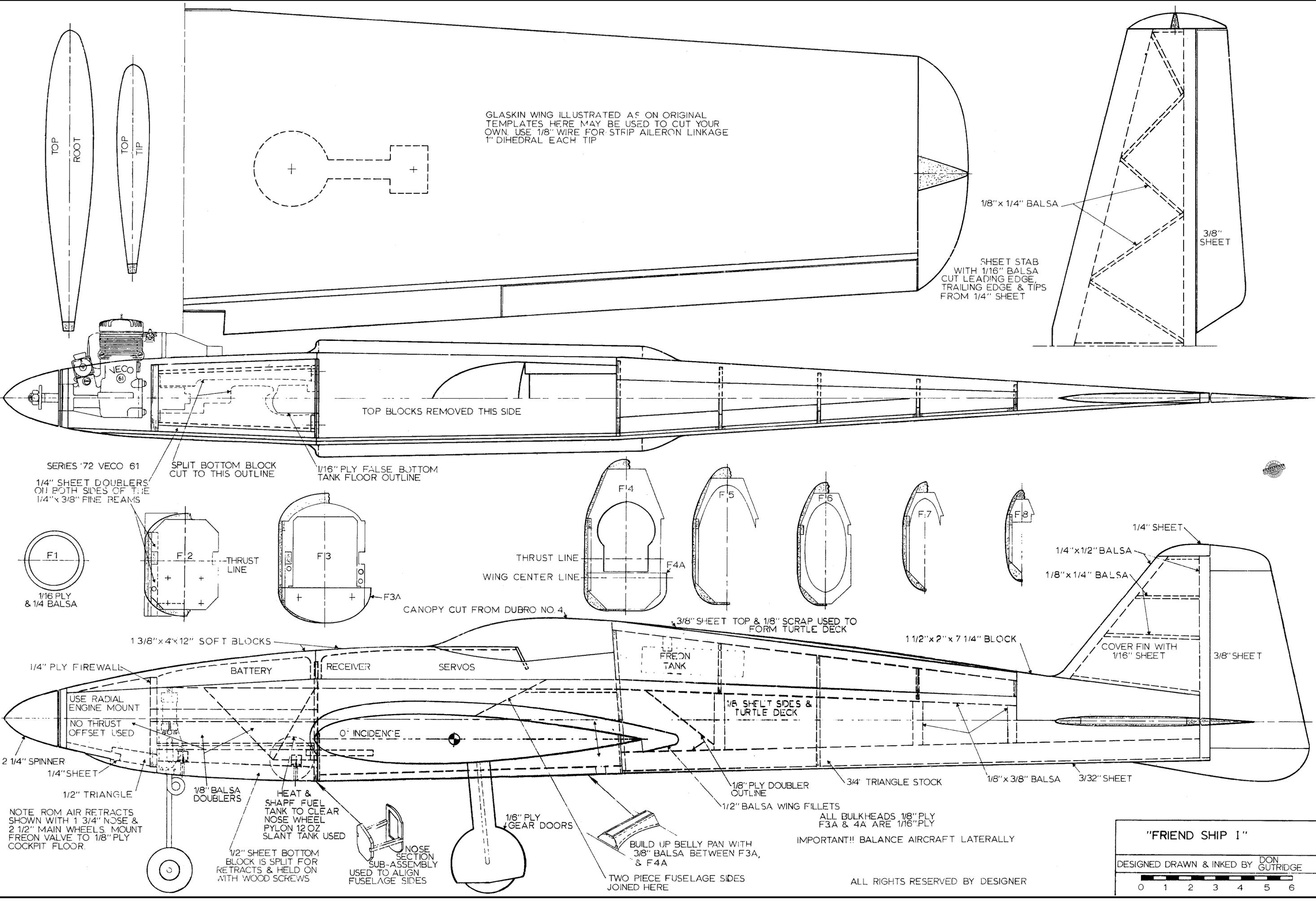
GLASKIN WING ILLUSTRATED AS ON ORIGINAL TEMPLATES HERE MAY BE USED TO CUT YOUR OWN. USE 1/8" WIRE FOR STRIP AILERON LINKAGE 1" DIHEDRAL EACH TIP
