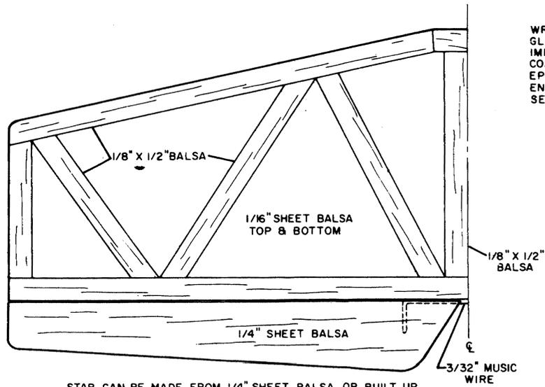
WRAP 4" WIDE GLASS CLOTH IMPREGNATED & COATED WITH EPOXY AROUND ENTIRE CENTER SECTION.
