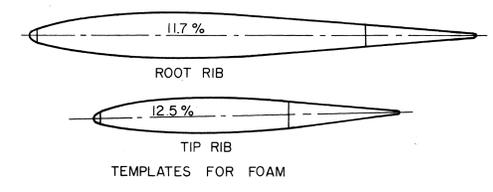
PLANE USES FOAM WING AND STAB COVERED WITH 1/64" PLYWOOD. FOR THOSE WANTING THE BUILT UP TYPE USE THE STACK METHOD.
